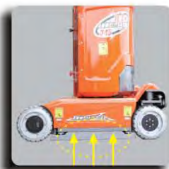
Automatic Pothole Protection
